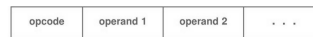
Figure 5.1 The general instruction format that many processors use. The opcode at the beginning of an instruction determines exactly which operands follow.
