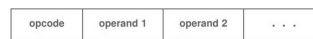
Figure 5.1 The general instruction format that many processors use. The opcode at the beginning of an instruction determines exactly which operands follow.
